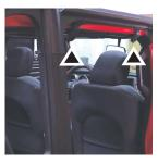
1. Remove the soft top support pillar. Unscrew the 2 screws on the roll bar and take the pillar away
