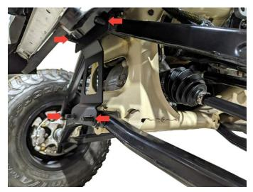
Remove the 4x 18mm factory control arm nuts that mount the bumper itself and then remove the bumper from the vehicle, install the supplied gusset plate onto the stud's paying attention to the offset of the plate facing the rear of the vehicle when installing.
