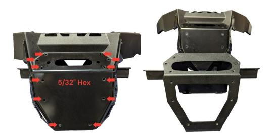
• Separate the inner structure from the outer bumper by removing the hardware with arrows pointing to them with a 5/32" hex tool and set the outer bumper aside for now.
