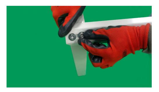
Use the wrench and 2x M8 nuts+washers to securely fasten into place, for each of the 4 corners
