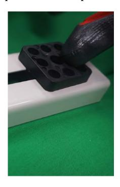
Step 7: Place the horizontal legs onto the frame and fasten using 4x M8\*16 bolt+nut/washer.
