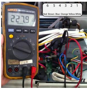
**2.** Turn off the power, and use a digital tester to measure the valve's resistance. The value should be  $1.8 \sim 2.5 \text{ K}\Omega$ .
