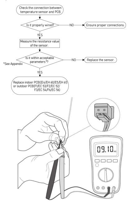
Note: For certain models, outdoor PCB cannot be removed separately. In this case, the outdoor electric control box should be replaced as a whole. This picture and the value are only for reference, actual appearance and value may vary. For certain models, outdoor unit uses combination sensor (T3, T4 and TP are the same of sensor).
