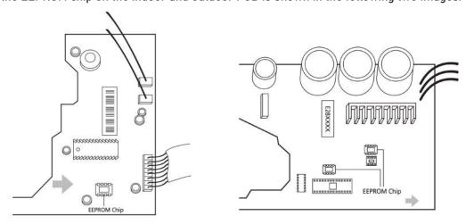
Note: For certain models, outdoor PCB cannot be removed separately. In this case, the outdoor electric control box should be replaced as a whole. This pictures are only for reference, actual appearance may vary.
