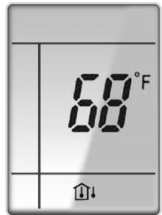
Room Temperature Display
