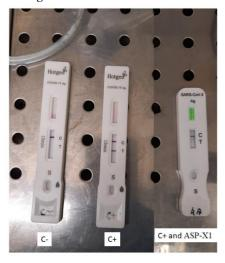
This experiment demonstrates that the Aurabeat Technology ASP-X1 equipment tested is able to completely neutralize the airborne viral load of SARS-CoV-2. In the experiment, the value of the PCR cycle turned negative compared to the non-purified sample, which had a value of 23 (viral nucleic acid) and 28 (Infectious intracellular viral load).
