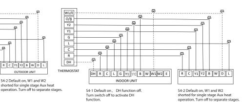
• Wiring for 3H and 1C thermostat
