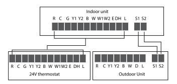
When using a 24V thermostat, please refer to the non-communicating wiring diagrams that follow:
