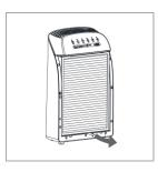
Pull out the composite filter element by the handle at the bottom of the filter.
