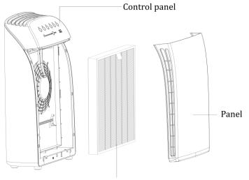
HEPA plus activated carbon composite filter
