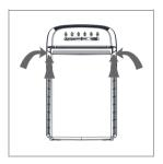
Reinstall the panel and lock the panel by pressing both sides of the top of the panel. After replacing the filter, plug the power cord back into an electrical outlet. Hold down the reset button for 3 seconds to reset the filter timer. The indicator light will flash 3 times and then go out, showing the reset was successful. (See Page 8)
