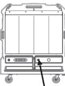
Fill the tank or attach a water hose. We recommend using the hose attachment with an automatic shut-off valve.
