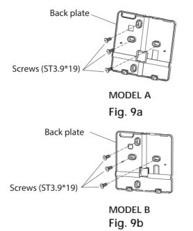
b. For flush mounting, fasten the back plate to the switch box with 2 screws (M4×25), and fasten the back plate to the wall with 1 screw (ST3.9\*19).
