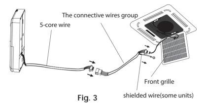
NOTE: Be sure to reserve a length of the connecting wire for periodic maintenance. If there is a connection lug at the end of shielded wire, the connection lug should be properly grounded.
