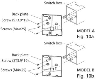
**NOTE**: Place the unit on a flat surface. Be careful not to distort the back plate of the remote control by over tightening the screws.
