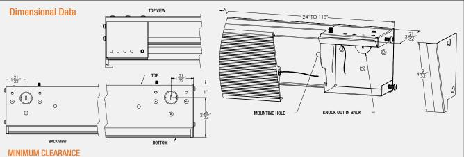
Heaters are not to be mounted closer than 21/2" from drywall ceiling or 6" from vinyl or drop ceiling. Heaters to be mounted at least 6 feet from floor.
