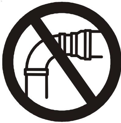
NO TRANSITION ON HORIZONTAL PLANE, THIS CREATES A WATER TRAP AND RESTRICTS FLUE GASES
