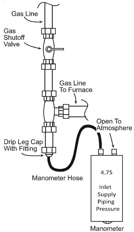
Measuring Inlet Gas Pressure (Alt. Method)
