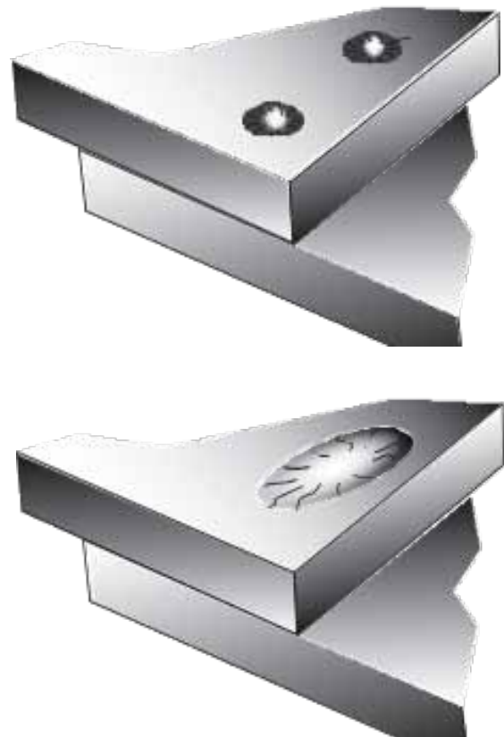
Plug Welds (Fig 1-19j)
