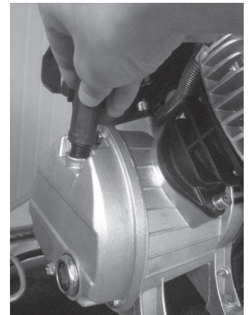
2. Check that the small hole in the top of the breather pipe is clear and then insert it into the oil filler hole.
