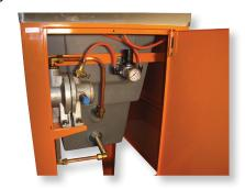
Solvent recycles well above the bottom of the tank. This allows the sludge to settle. Water can be filled to just below the outlet and this will keep the solvent cleaner.
