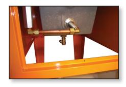
Safety control valve stops machine unless lid fully closed.
