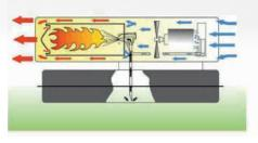
Combustion system - air flow
