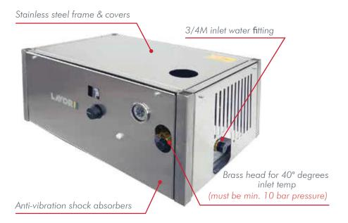
Three phase ultra powerful cold water pressure washer suited for the most industrial environments. Powerful 21L/min@2900psi will shift the most stubborn dirt grease or muck. Featuring water cooled 1450 RPM slow speed motor/pump, delayed Total Stop and stainless protection, the MCHPX series is tough as nails.
