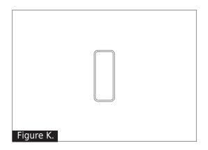
If the ladder side-rail is a Rectangular shape, it does not require the aluminium spacer to be placed on the side-rail (Figure K).
