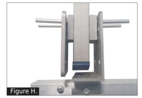
If the ladder side-rail is an I-shape, please place the aluminium profile spacers  $65 \times 45.8 \times 14$ mm on both sides of the rail. For each side of the rail, use 2 locating pins to hold the aluminium spacer in position (Figure G and Figure H).
