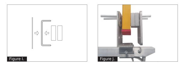
If the ladder side-rail is a C-shape, please place the aluminium profile spacers  $65 \times 45.8 \times 14$ mm and the aluminium profile spacers  $127 \times 50 \times 1.5$ mm on the rail (Figure I and Figure J).
