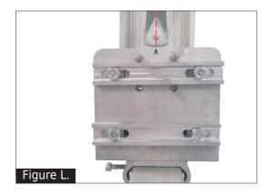
3. Make sure the bolts sit tightly against the side-rail. Place aluminium spacers, ladder foot clamp B, bolts, nuts and washer back on both sides. Bolts are placed on 4 slot holes (Figure L).
