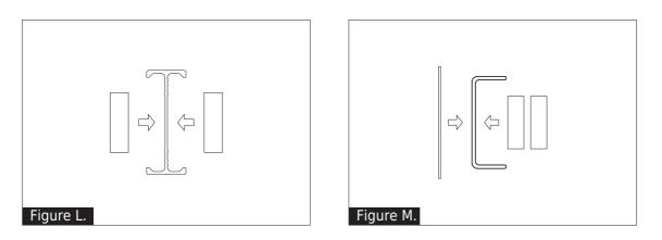
If the ladder side-rail is an I-shape, please place the aluminium profile spacer 65 x 45.8 x 14mm on both sides of the rail (Figure L).
