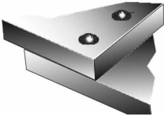
Plug Welds (Fig 1-19j)
