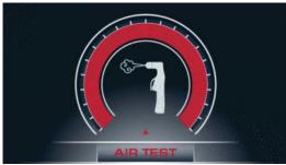
Long press button(8) for 2 seconds to enter the check gas, and the display screen will display the above interface
