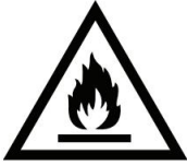
RISK OF FIRE
