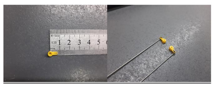
Set aileron servos horns 30-40 degrees back at neutral servos position.
