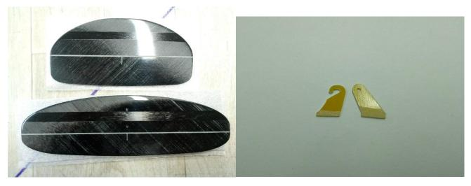
Avoid contact of superglue with foam of the wing and tail cores! Paste in control horns using epoxy.
