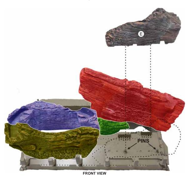
Place the Top Middle Log (F) into the right recess on the Back Left Log (C) and the left end of the Right Front Log (E).
