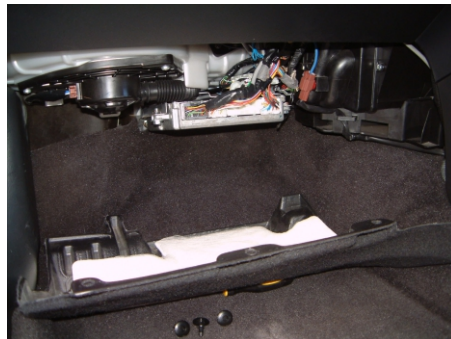
Figure 2 - Removing Glove Compartment
