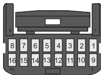
AUXILIARY CONNECTOR (16 PIN) REAR VIEW (WIRE SIDE)
