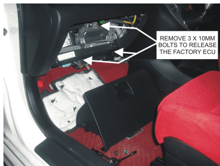
Figure 3 - Removing the factory ECU
