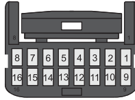
AUXILIARY CONNECTOR (16 PIN) REAR VIEW (WIRE SIDE)
