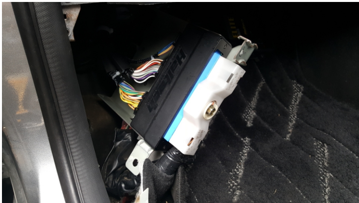
Figure 3 - Typical Plug 'N' Play Adaptor installation (Double-sided tape aybe used to secure the Adaptor to the factory bracket)
