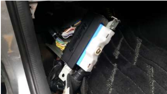
Figure 3 - Typical Plug 'N' Play Adaptor installation (Double-sided tape maybe used to secure the Adaptor to the factory bracket)
