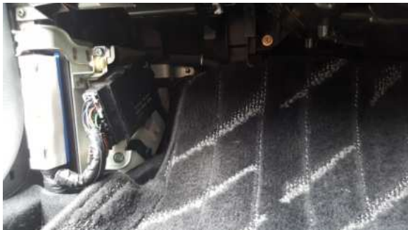
Figure 4 - Final installation should look like this with ECU secured under the carpet
