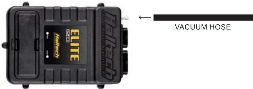
Figure 1 - Elite ECU internal MAP sensor
