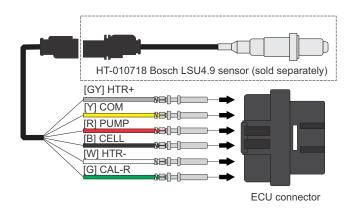
WARNING: Check your ECU's quick start guide for the pins used for onboard wideband control. Incorrect installation of this wideband sensor kit WILL damage your ECU.
