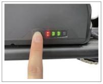
♦ Use the charger with the corresponding voltage and current, insert the DC plug of the charger into the battery, and insert the power plug into the mains socket.the charger light shows red when it is charging, and green when it is fully charged.
