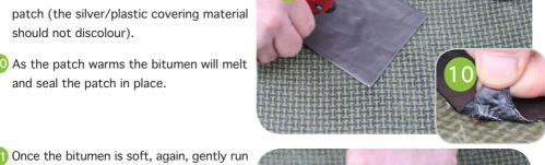
a hard, rounded edge (edge of blowtorch, knife sheath), across the patch to apply pressure and seal it in place.
