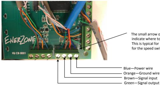
The small arrow on the board will help indicate where to position the first wire This is typical for each terminal connector for the speed switch..
