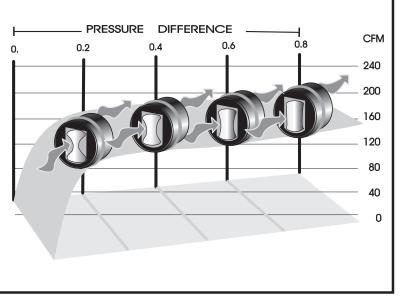
**CAR Airflow Performance Data:** Performance charts reflect airflow measurements taken at 68° (20° C) at 1 atmosphere pressure. CAR's designed for system pressures above 0.8 in. w.g. are also available. Consult the factory for information.
