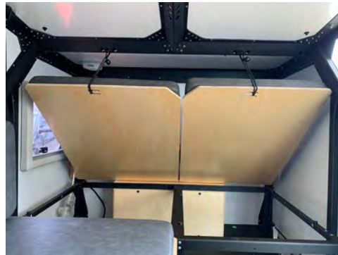
Group 24 Battery shown (not included) Space for second battery (Group 24 or 27 fits)
