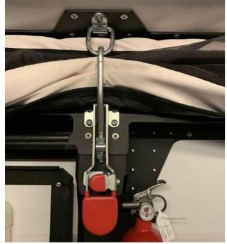
2. Push roof up from center front of roof interior. Place hands on either side of center spine and push upwards. Gas springs will assist the lift and prevent a sudden closing.
