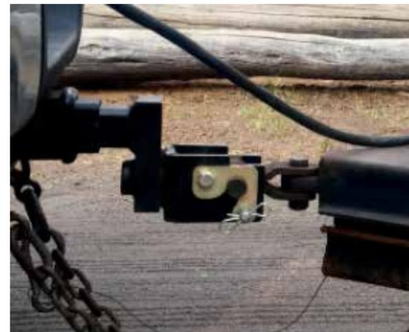
1. Crank the tongue of the habitat jack until the hitch coupler is raised enough to clear the tow vehicle;
