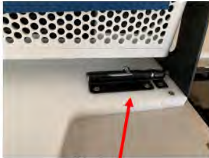
With exterior AC shroud in up position, unlock both sides and push AC into operating position
