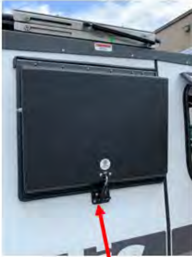
AC shroud shown in locked / driving position
