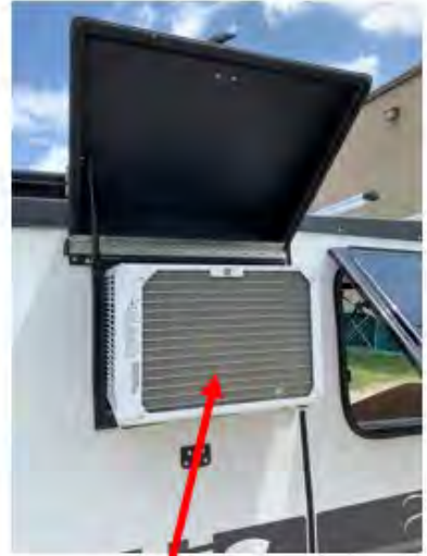
AC shroud shown open and with AC in pushed out / operating position
