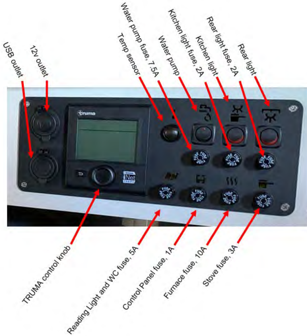
FUSE AND SWITCH PLATE AT KITCHEN
