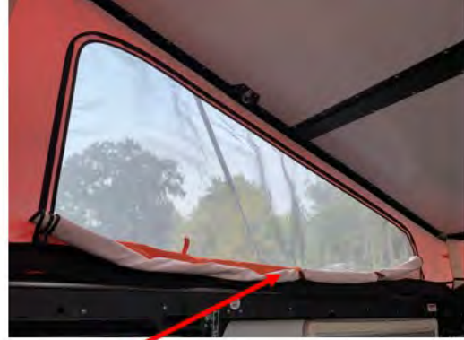
If all the way open Use toggles to make neat (close during driving rain!!)
