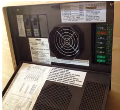
WFCO power center
