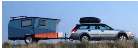
proper ~10 to 15% of habitat on car coupler and or introduction of 'weight distributing' hitch system
