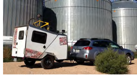
proper ~10 to 15% of loaded trailer on tongue
