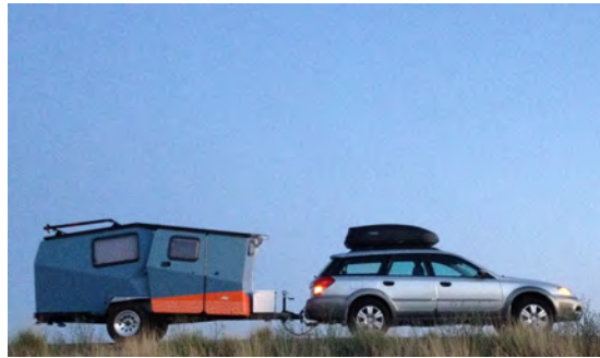
proper ~10 to 15% of trailer on car coupler
