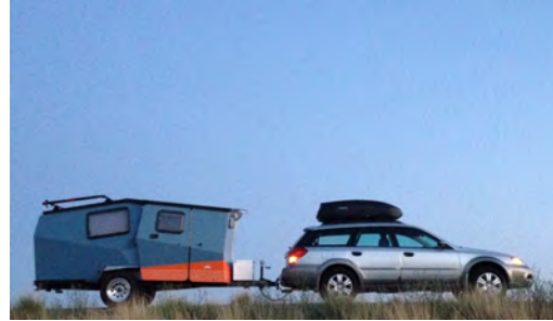
proper ~10 to 15% of trailer on car coupler
