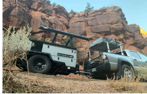
proper ~10 to 15% of loaded trailer on tongue
