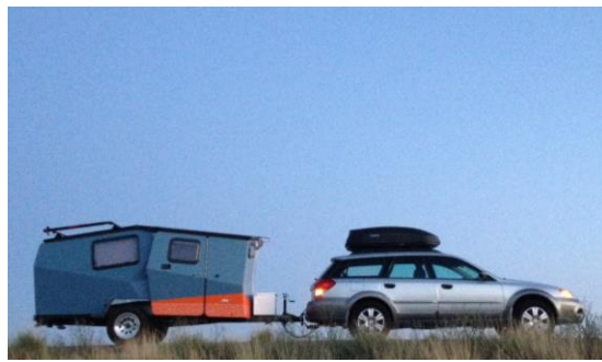
proper ~10 to 15% of trailer on car coupler
