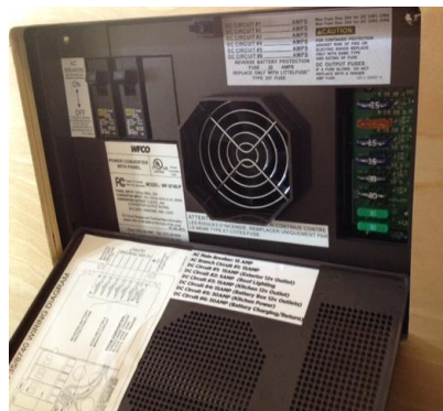
WFCO power center
