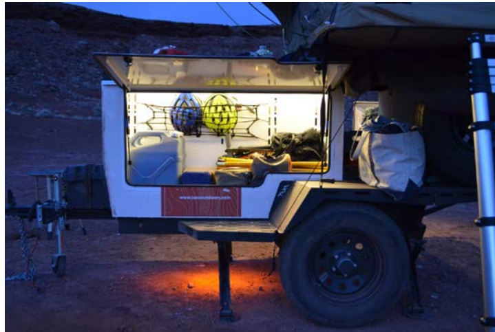
cargo bay – attach points for nets and tie downs, night lighting
