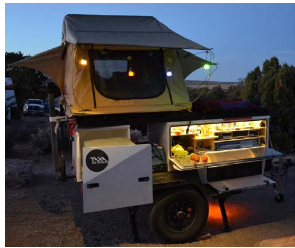
kitchen / workspace – night lighting, switches and USD outlets, cargo beneath
