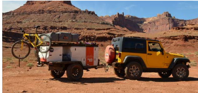
proper ~10 to 15% of loaded trailer on tongue
