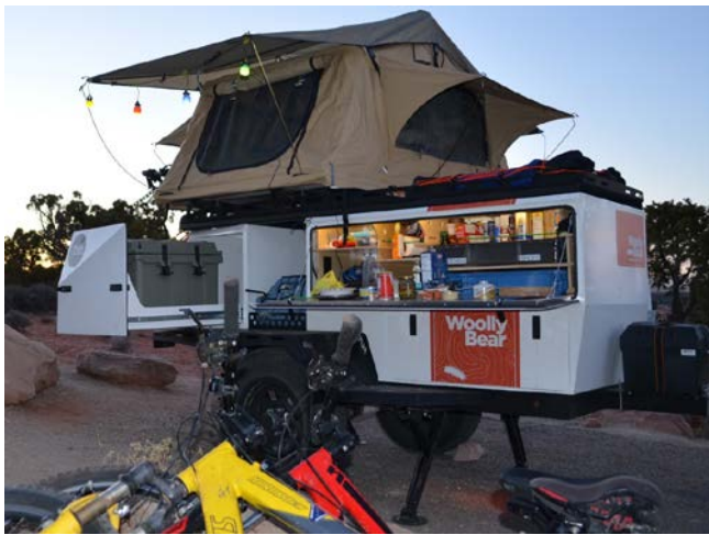
kitchen / workspace – night lighting, switches and USD outlets, cargo beneath
