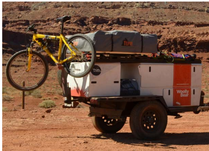
cargo deck – integrated tie down point, 5 locations for load bars allows multiple load arrays for usage or weight distribution
