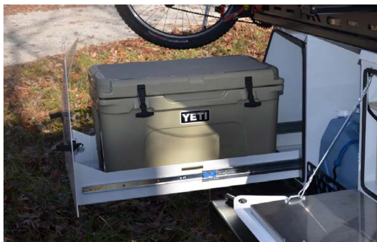
cargo drawer – cooler (YETI 45 quart shown), tie down slots and cooler drain in drawer bottom
