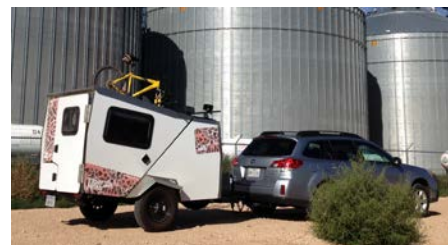
proper ~10 to 15% of loaded trailer on tongue
