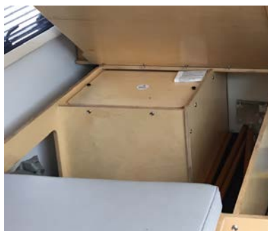
Battery compartment beneath Couch
