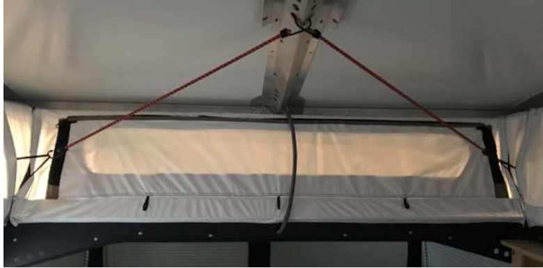
SHOWS REAR OF ROOF, OPEN POSITION, BUNGEEES HELP PULL TENT IN WHEN CLOSING
