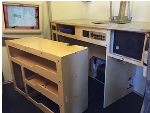
(shows kitchen with shelf unit detached and pulled away for access to plumbing and wiring innards. Unit detaches / attaches with three wingnuts)
