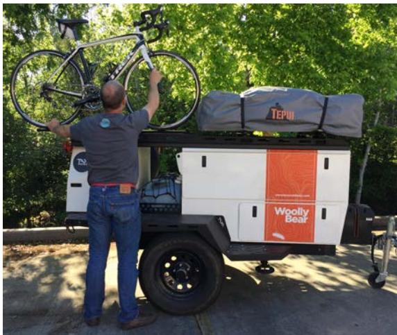
cargo deck – integrated tie down point, 5 locations for load bars allows multiple load arrays for usage or weight distribution
