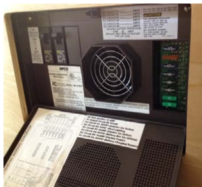
WFCO power center
