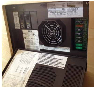
WFCO power center
