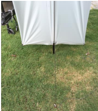
3 stake pattern (front pole, 2 bottom corners)
